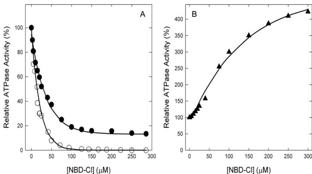
FIG. 4. Effect of NBD-Cl on  $\beta$ N243A and  $\beta$ N243D mutant  $F_1$  ATPase activity. Purified  $F_1$  was preincubated 60 min at 23 °C with varied concentrations of NBD-Cl and then assayed for ATPase activity. For details, see “Experimental Procedures.”  $\circ$ , wild type;  $\bullet$ ,  $\beta$ N243A;  $\blacktriangle$ ,  $\beta$ N243D. Data are means of at least quadruplicate experiments. Variation was  $\pm 10\%$  between different experiments.
