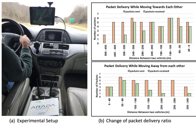
Figure 1: (a) OBU inside the vehicle (b) Packet delivery ratio at 55 mph
