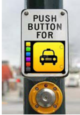
Figure 4.4: Roadside Hailing Device for taxi calling
