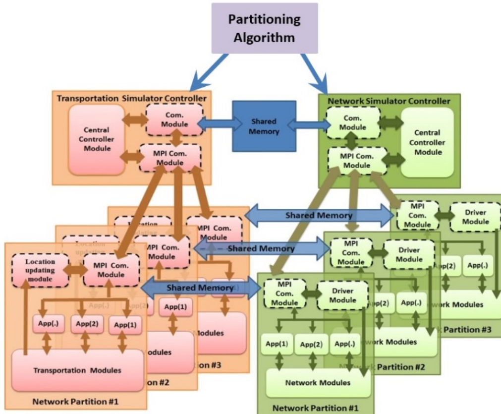
Figure 4. Envisioned distributed simulation architecture incorporating hybrid parallelism
