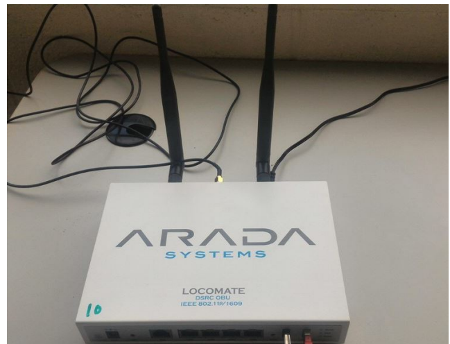
Fig. 2: ARADA On Board Units used for test.
