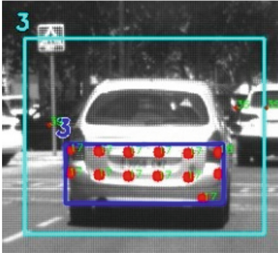
Fig. 6. Obstacle detection based on cluster computation.
