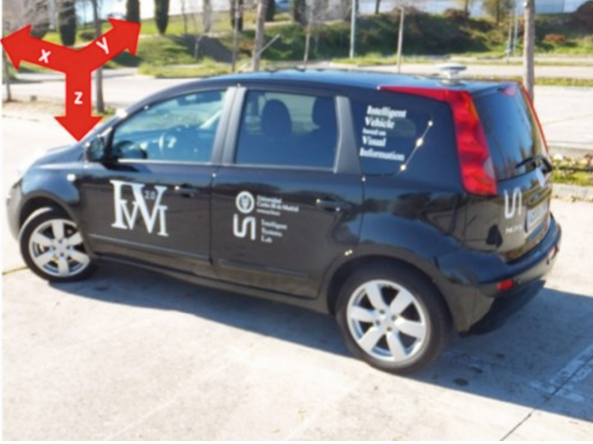
Fig. 3. IVVI 2.0 research platform with axis represented in the image: X = laser-obstacle distance, Z = detection height, Y = horizontal deviation from the laser.
