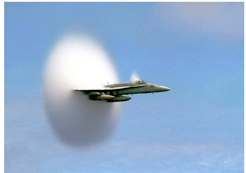
Here a jet goes supersonic leaving behind a condensation cloud.
