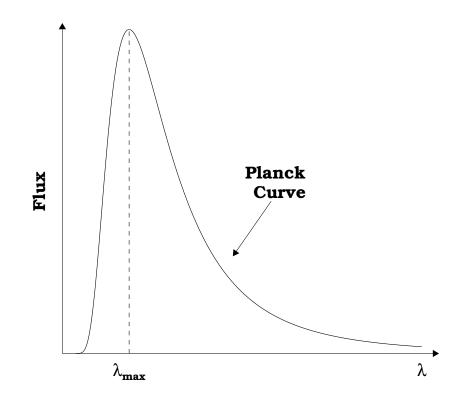
d) The energy flux (F) is the amount of energy emitted from each square meter of an objects surface per second. The flux of a blackbody is a function only of its temperature and is given by the **Stefan-Boltzmann law**:
