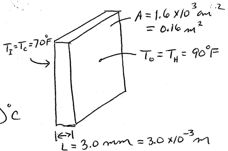
$$P_{\text{cond}} = \frac{\Delta Q}{\Delta t} = \frac{k A \Delta T}{L} = \frac{(0.8 \frac{\text{J}}{\text{m} \cdot \text{C}}) (0.16 \text{ m}^2) (11.1^\circ \text{C})}{3.0 \times 10^{-3} \text{ m}}$$
