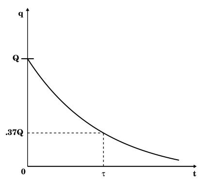
c) Note that the capacitor is now acting like a battery, however, a battery with a continually decreasing voltage:
