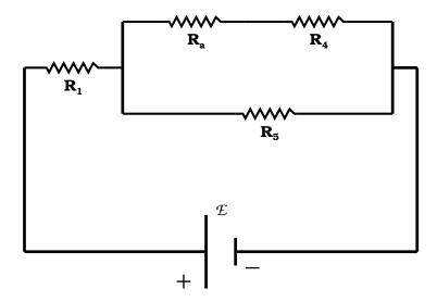
We see from the diagram above that we now need to reduce the 2 series resistors  $R_a$  and  $R_4$  with Eq. (IV-5) giving
