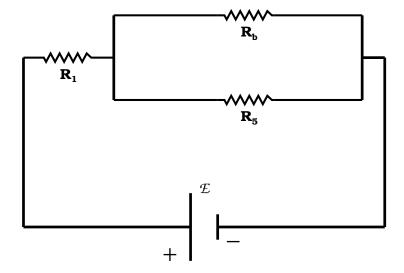
The diagram below show the next stages on route to the final equivalent resistor: Reduce the parallel  $R_b$  and  $R_5$  resistors followed the series  $R_c$  and  $R_1$  resistors as shown in the next diagram.
