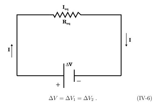
2. The current entering a parallel circuit is equal to the sum of all currents traveling through each resistor:
