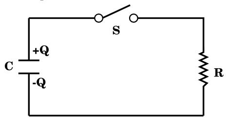
a) When we close the switch, the capacitor begins to drain following:
