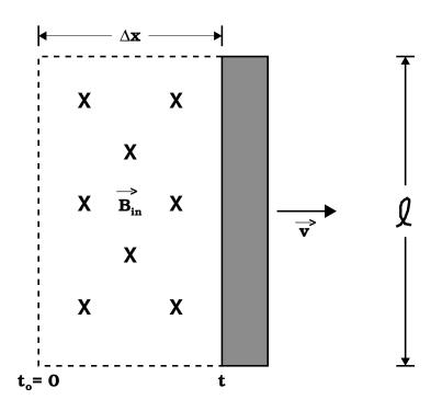
a) As the bar moves, the magnetic flux increases:
