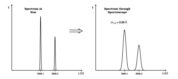
ii) A low-resolution spectrograph has  $\Delta \lambda_{1/2} > 0.1$  Å. An example of a low-resolution spectrum is shown below.
