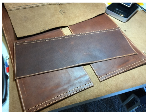
The top and ends of the bag. I had just finished punching these holes. Next, stitching.
