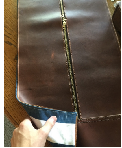
Right before stitching the brass zipper in, seen here. This is the top of the bag.
