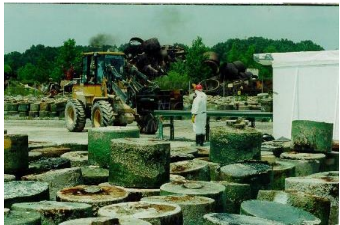
Several thousand tons of nickel and aluminum ingots were produced. These materials are currently stored outside with no protection.
