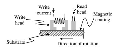
Data Encoding: It might seem natural to use the two directions of magnetic polarization to represent 1's and 0's. This is not the case for two reasons.
