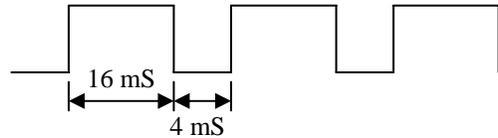
First, be sure to use the correct value for the period, i.e., it is one full cycle of the signal from high to low and back to high. This becomes  $16 \text{ mS} + 4 \text{ mS} = 20 \text{ mS}$ . Next, we need to invert the period in order to calculate the frequency.
