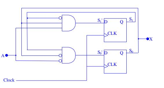
$S_0' = \overline{S}_0 S_1 \overline{A}$   $S_1' = S_0 \overline{S}_1 A$   $X = S_0$
