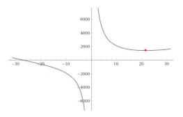
The minimum (marked with the dot) occurs at some value slightly less than x=22 inches.
