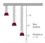
**Solution.** Since the position  $s = 5 \cos t$ , then the velocity is  $v = ds/dt = -5 \sin t$  and the acceleration is  $a = dv/dt = -5 \cos t$ .
