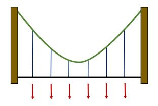
We cut the cable at its lowest point and at a point a distance x from the lowest point:
