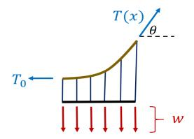
Let  $T_0$  be the tension at the lowest point and let T(x) be as in the picture. Then from the example equations:
