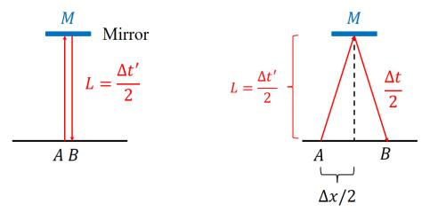
In S, the light returns to the origin (x' = 0) at time  $t = \Delta t = t'/\sqrt{1-\beta^2}$  (equation (78), page 123). Also, in S with x' = 0 we have (from equation (86)) that  $t = a_{44}t'$ . Therefore  $a_{44} = 1/\sqrt{1-\beta^2}$ . Next, with x' = 0 and  $t = t'/\sqrt{1-\beta^2}$ , since the point x' = 0 occurs in the S frame at  $x = \beta t$  (due to the relative motion), we have from
