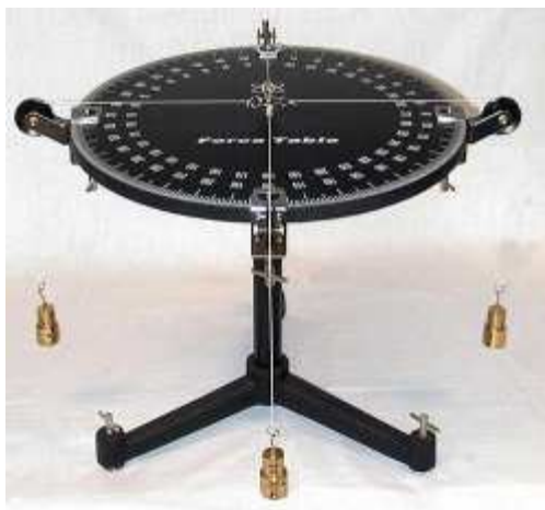
Figure 8: A force table similar to the ones used in this class.
