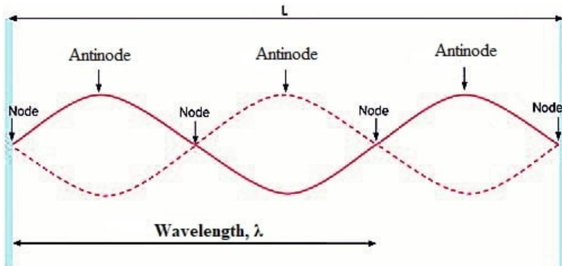
Figure 1: Stationary Wave on a String
